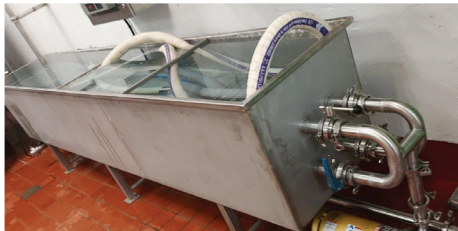
HOSE CIP UNIT
