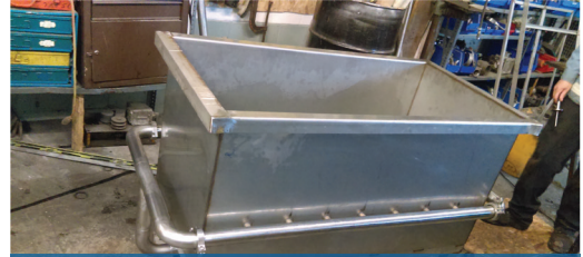
DESIGN MANUFACTURED NEW CLEAN-IN-PLACE (CIP) UNIT
